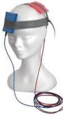
Figure 3.1. Depiction of the electrode montage used in both Study 1 and Study 2. The red (upper) sponge represents the anodal electrode placed over the left primary motor cortex and the blue (frontal) sponge represents the cathode placed over the right supraorbital ridge.
